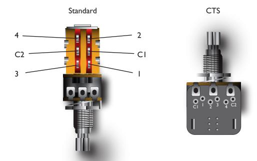
Switch pulled UP - C1 connects to 1, C2 connects to 3 Switch pushed DOWN - C1 connects to 2, C2 connects to 4
