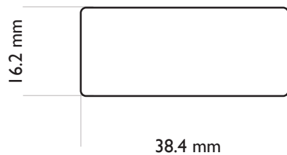
8 STRING SOAPBAR WIDTH & HEIGHT DIMENSIONS (BRIDGE & NECK)
